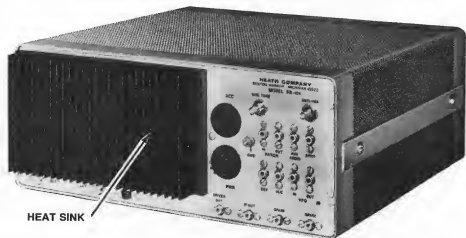
Figure 3-25 The heat sink on a 100 watt solid state amateur radio transceiver.
